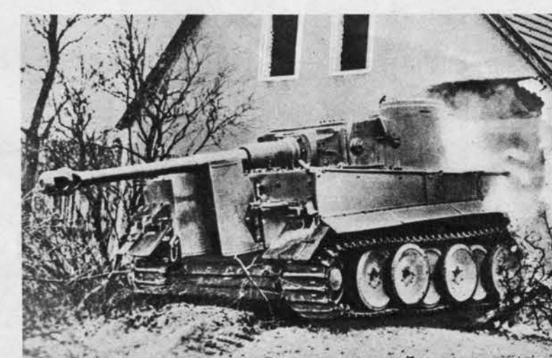
Nazi propaganda picture advertises the ramming technique of their 62-ton Tiger tank. This rear view, with the 88-mm. gun reversed, illustrates the Tiger's wide track, large idler and flat, overlapping wheels.
